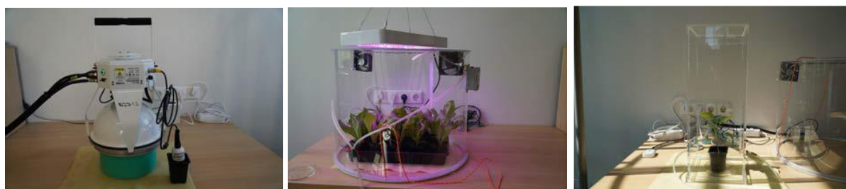
Figure 11. Gas flux measurement chambers for measuring soil respiration and ecosystem respiration (Re; left photo), and photosynthesis and net ecosystem gas exchange (Net Ecosystem Exchange NEE) (middle and right photos).
